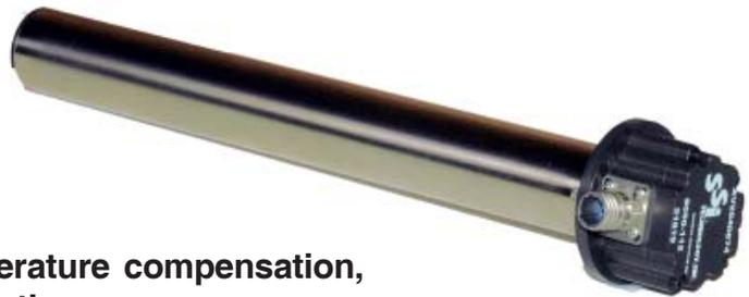
The SSI FG-2400 Fuel Level Monitoring system is a microprocessor based solid-state capacitive (no moving parts) gauging device for measuring the remaining fuel. Its capacitive probe is an integral part of the flange-gauge assembly. This sensor was designed to measure fuel tanks in excess of 5,000 gallons, while maintaining an accuracy of +/- 5%. Higher accuracies are attainable on a tank to tank basis.
